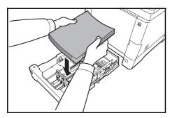
5 Load the paper in the cassette. Ensure the side to be printed is facing up and the paper is not folded, curled, or damaged.
